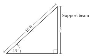
What is the height (h) of the beam that is needed to support the roof? Round the answer to the nearest foot.
